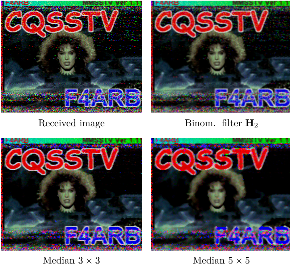
Figure 13.9: The results of noise reduction with median filter.
